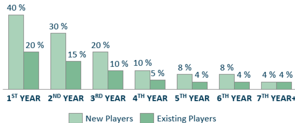
Figure 30a: MODELING - SCRAP RATE PER PLAYER TYPE AND YEAR OF PRODUCTION | %, Through the Factory Production Life
